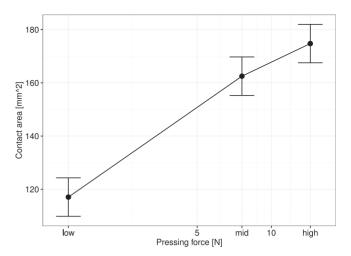
Fig. 4. Contact area as a function of pressing force in the sinusoidal vibration condition. Error bars  $\pm SE$ .
