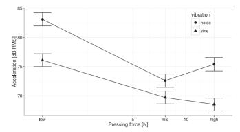
Fig. 2. Thresholds measured at three pressing force levels, for sinusoidal and noise vibrations. Error bars  $\pm \rm SE$ .
