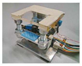
Fig. 1. The touch-box: The interface used in the experiment to yield vibrotactile feedback and to measure finger force and contact area.
